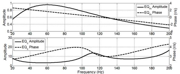
Figure 4.5 Amplitude (solid line) and phase (dotted line) values of the calculated microphone (top) and subwoofer (bottom) filter coefficients for  $G_d = 9$
