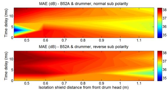
Figure 3.9 Mean absolute error (MAE) measurements between the drummer and microphones for variable electronic time delay and isolation shield position
