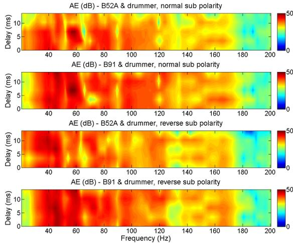
Figure 3.8 Absolute error (AE) measurements between the drummer and microphone references for variable electronic time delay versus frequency
