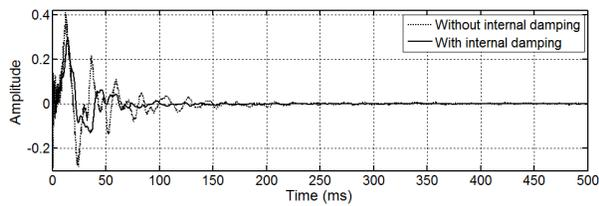
Figure 3.6 B52A measured responses with (solid line) and without (dotted line) internal kick-drum damping (no subwoofer/isolation shield)
