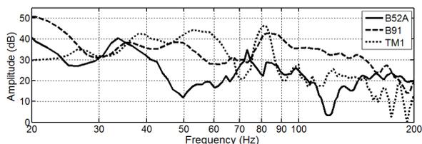
Figure 3.2 Reference kick-drum frequency responses (no subwoofer/isolation shield)
