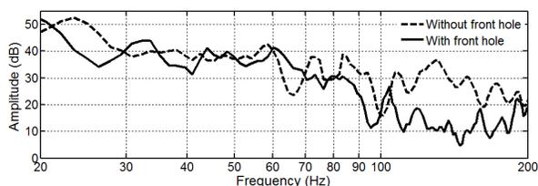
Figure 3.3 B52A measured frequency responses with (solid line) and without (dotted line) a front head hole (no subwoofer/isolation shield/internal damping)
