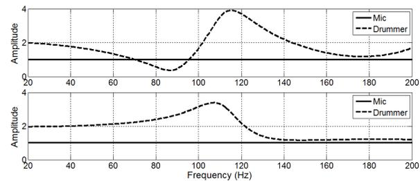
Figure 4.8 Corrected microphone and drummer frequency responses for a drummer position offset of 50 cm (top) and -50 cm (bottom)
