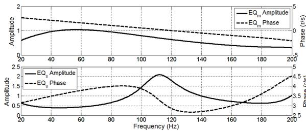
Figure 4.4 Amplitude (solid line) and phase (dotted line) values of the calculated microphone (top) and subwoofer (bottom) filter coefficients for  $G_d = 1$
