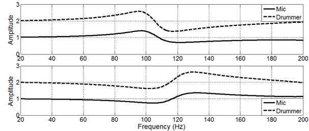
Figure 4.7 Corrected microphone and drummer frequency responses for a microphone position offset of 10 cm (top) and -10 cm (bottom)
