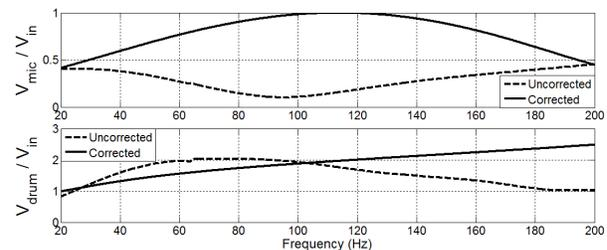
Figure 4.8 Simulated uncorrected (dotted line) and corrected (solid line) transfer functions for the microphone and drummer position
