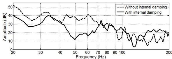
Figure 3.5 B52A measured frequency responses with (solid line) and without (dotted line) internal damping (no subwoofer/isolation shield/internal damping)
