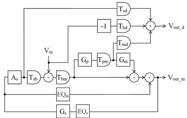
Figure 4.1 Comprehensive optimization system configuration for kick-drum/subwoofer/isolation shield setup utilizing subwoofer EQ and echo-cancellation
