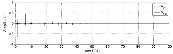
Figure 4.6 Generated subwoofer signal (solid line) due to a Dirac delta function input (dotted line at  $t = 0$  ms)
