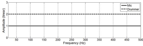
Figure 4.3 Theoretical corrected frequency responses at the microphone (solid line) and drummer (dotted line)
