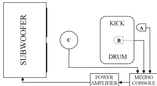
Figure 3.1 Measurement setup for kick-drum and drum subwoofer system (A = B52A, B = B91, C = TM1)
