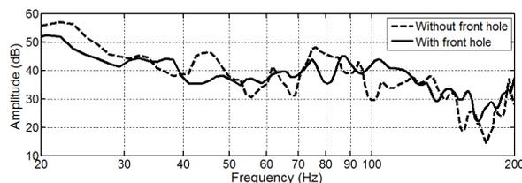
Figure 3.4 B91 measured frequency responses with (solid line) and without (dotted line) a front head hole (no subwoofer/isolation shield/internal damping)
