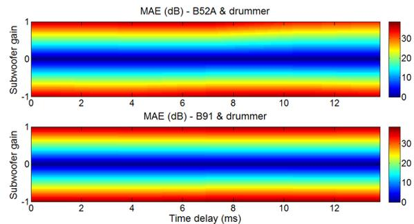
Figure 3.7 Mean absolute error (MAE) measurements between the drummer and microphone references for variable subwoofer gain and electronic time delay
