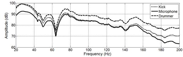
Figure 4.7 Simulated frequency responses for the drummer position (dashed line) and microphone (solid line) as compared to the dry B52A kick-drum measured frequency response (dotted line)
