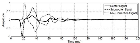
Figure 4.6 Generated subwoofer (dashed line) and microphone correction (dotted line) signals using the dry B52A kick-drum measurement (solid line)
