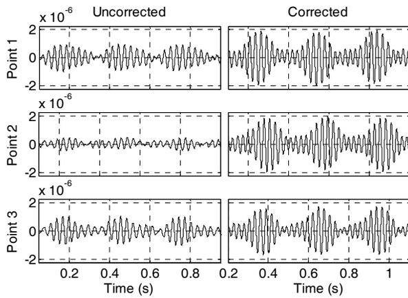
Fig. 3.7 Tone-burst measurements (34.7 Hz) at three locations using system configuration A
