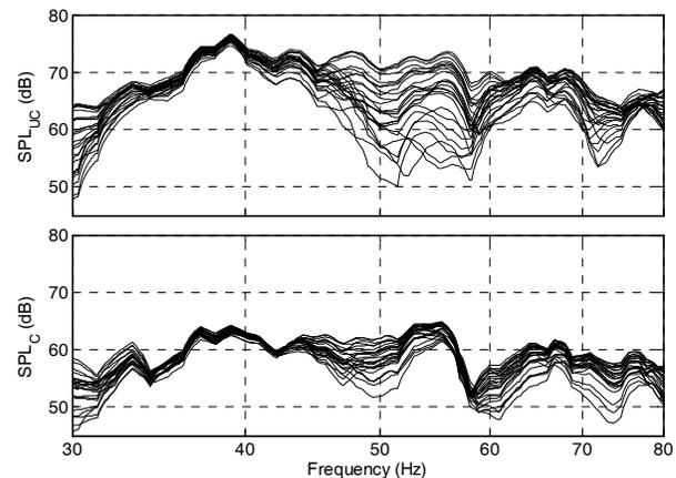
Fig. 3.5 Uncorrected (top) and corrected (bottom) frequency responses over a 25-point walking path using system configuration C
