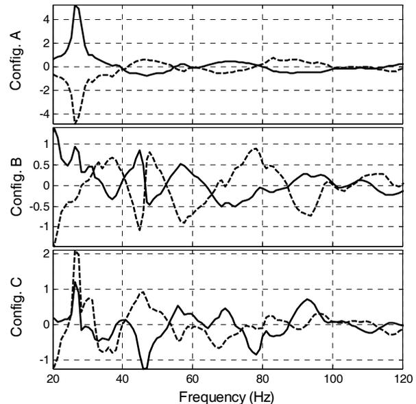
Fig 3.1 CSA correction filter frequency responses for configurations A, B and C (solid line = subwoofer 1, dashed line = subwoofer 2, linear amplitude scale)
