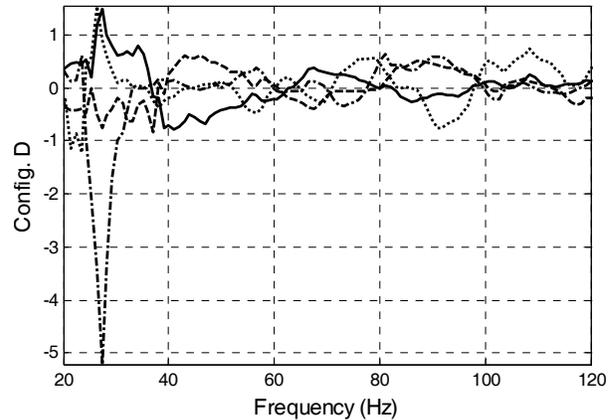
Fig. 3.13 CSA correction filter frequency responses for configuration D (4 subwoofers, linear amplitude scale)
