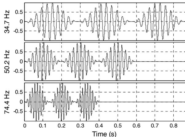
Fig. 3.6 Source tone burst waveforms (linear amplitude scale)
