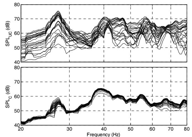
Fig. 3.14 Uncorrected (top) and corrected (bottom) frequency responses over a 25-point walking path using the four-subwoofer system configuration
