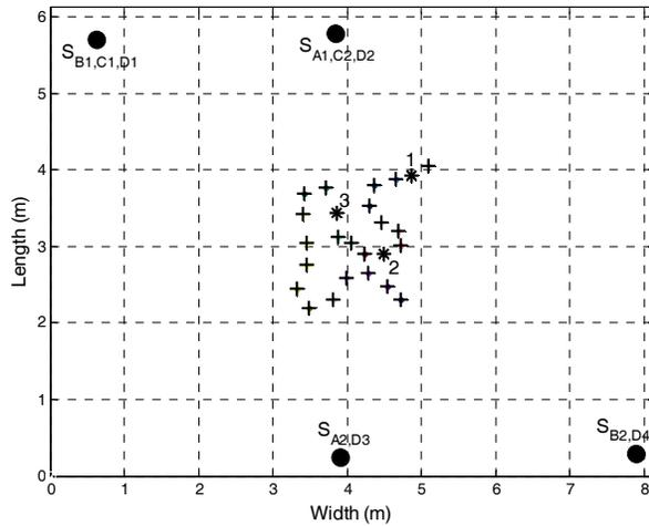
Fig. 3.2 Subwoofer configurations and 25-point walking path used for CSA performance evaluation (starred/numbered points indicate tone burst measurement points, as discussed in Section 3.2, configuration D discussed in Section 3.3)
