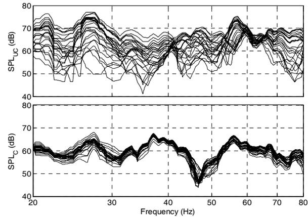
Fig. 3.4 Uncorrected (top) and corrected (bottom) frequency responses over a 25-point walking path using system configuration B
