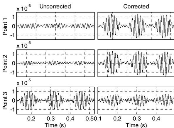
Fig. 3.9 Tone-burst measurements (74.4 Hz) at three locations using system configuration A
