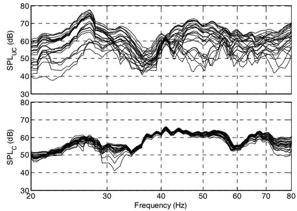
Fig. 3.3 Uncorrected (top) and corrected (bottom) frequency responses over a 25-point walking path using system configuration A
