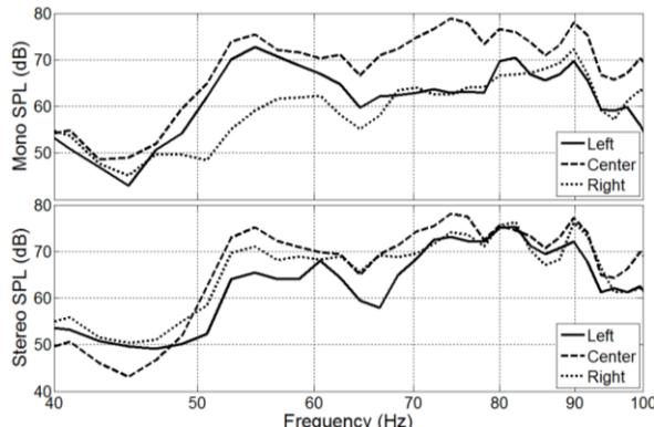
Fig. 4.2 Frequency responses for three measurement locations due to a mono (top) and stereo (bottom) subwoofer system (outdoor test space)
