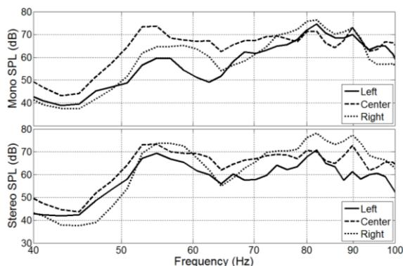
Fig. 4.4 Frequency responses for three measurement locations due to a mono (top) and stereo (bottom) subwoofer system (indoor test space)
