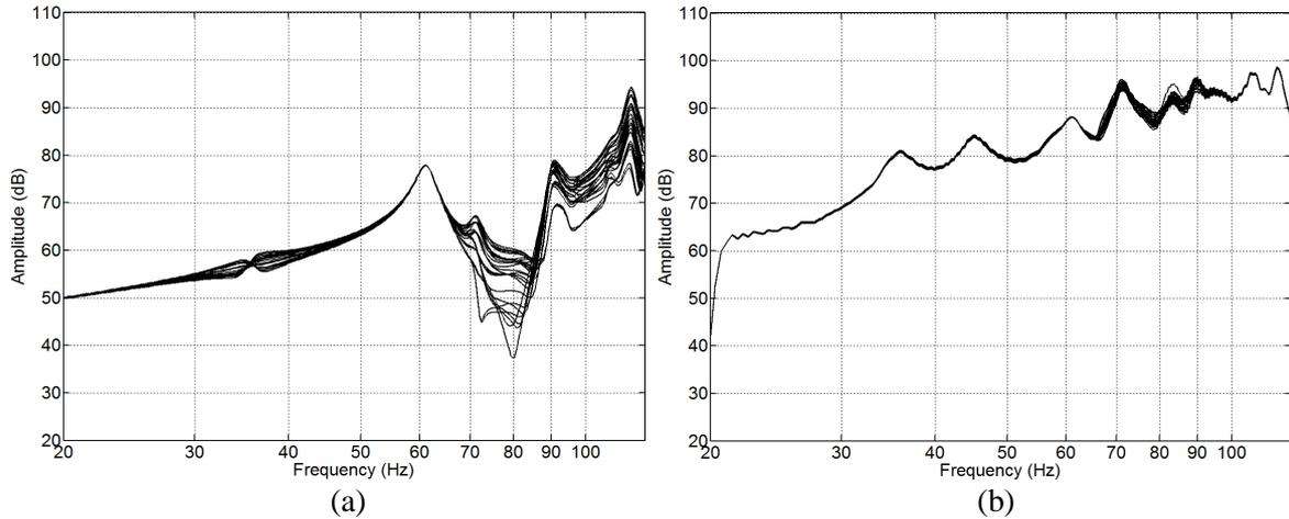
**Figure 2.** Frequency response at points along a virtual walking path for (a) four omnidirectional subwoofers at wall midpoints and (b) a four-unit CSA at wall midpoints
