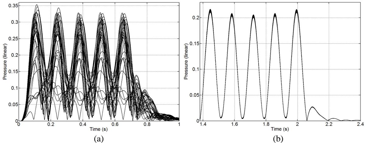
**Figure 3.** Simulated waveforms along a virtual walking path from 110 Hz tone burst simulation for (a) uncorrected system and (b) CSA corrected system
