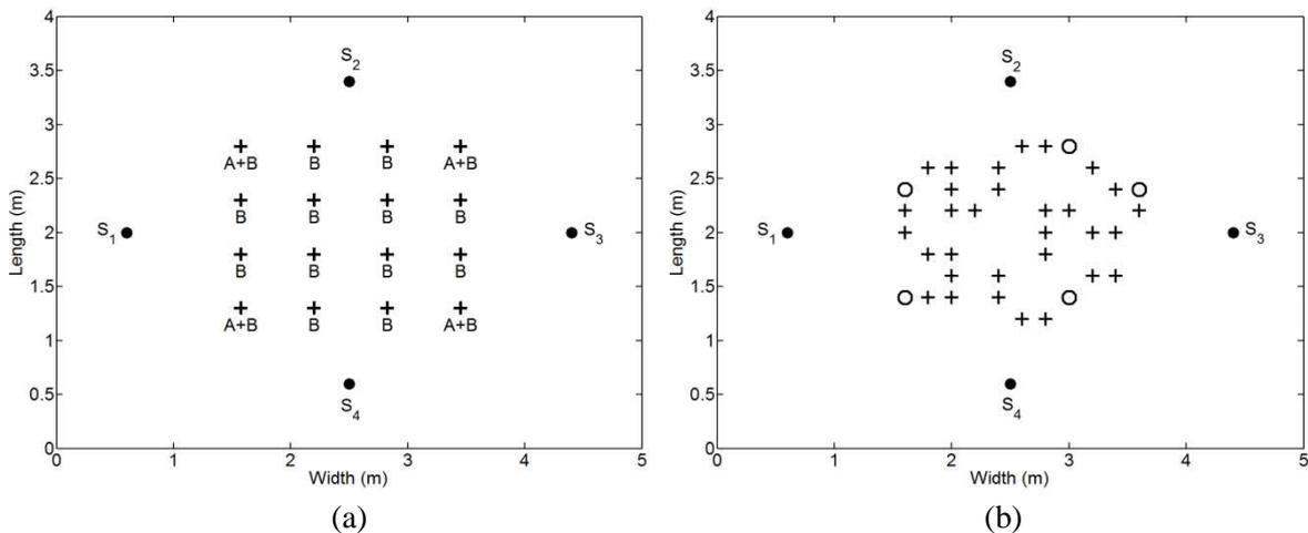
**Figure 1.** Four-unit layout for (a) CSA correction filter calculation (A = omni, B = omni + dipole) and (b) 36-point virtual walking test (circles = target points, crosses = non-target points)
