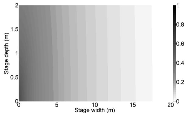
Fig 4.2 Received signal strength (RSS) map for an antenna (0.0 m, 0.0 m, 2.0 m) and calibration location (0.5 m, 0.5 m, 1.6 m), over the first 2 m of stage depth
