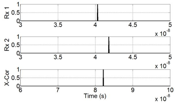
Fig 4.5 Example of cross-correlation based on received signals at two antennas located at (0.0 m, 0.0 m, 2.0 m) and (0.0 m, 5.0 m, 2.0 m) and a transmitter located at (12.0 m, 1.4 m, 1.6 m)
