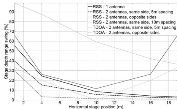
Fig 4.8 calculated range percentages for various horizontal locations using various system configurations (anechoic environment)
