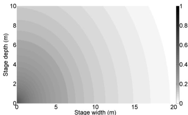
Fig 4.1 Received signal strength (RSS) map for a single antenna at (0.0 m, 0.0 m, 2.0 m) and a calibration location (0.5 m, 0.5 m, 1.6 m)
