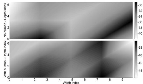
Fig 4.9 Received signal strength (RSS) measurements for two antennas at (0.7 m, 0.0 m, 2.0 m) and (9.1 m, 0.0 m, 2.0 m) with no human interference (top) and with human interference (bottom)
