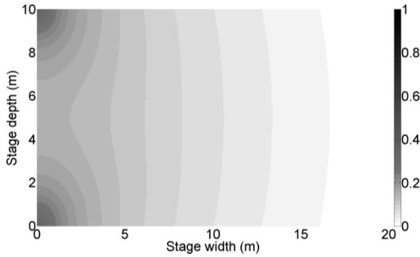
Fig. 4.4 Received signal strength (RSS) map for two antennas at (0.0 m, 0.0 m, 2.0 m) and (0.0, 10.0, 2.0), with calibration location (0.5 m, 0.5 m, 1.6 m)
