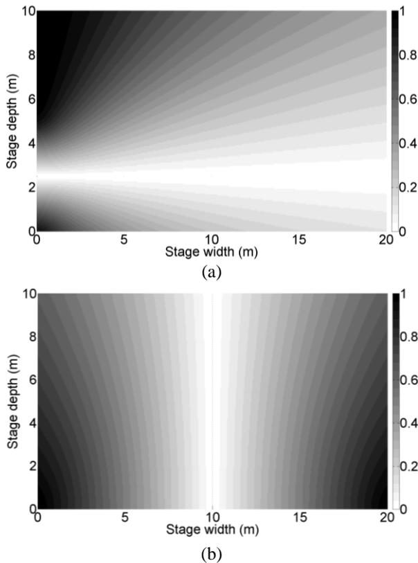
Fig. 4.7 TDOA map for two antennas at (0.0 m, 0.0 m, 2.0 m) and: (a) (0.0, 5.0, 2.0) or (b) (20.0, 0.0, 2.0)
