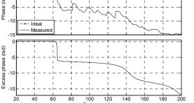
Fig. 3.3 Comparison of ideal and measured phase responses (top) and the excess phase components of the measured phase response (bottom)
