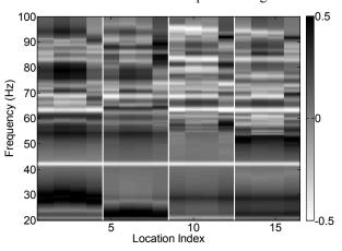
Fig. 3.14 Simulated error agreement as a function of frequency and location index, as a result of a two dipole subwoofer <sup>1</sup>/<sub>4</sub> sidewall length configuration
