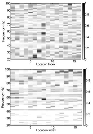
Fig. 3.6 Simulated MD (top) and PV (bottom) as a function of frequency and location index (see Fig. 3.5), as a result of a single corner subwoofer configuration
