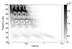
Fig. 3.2 Absolute error between direct and impulse response-derived tone burst measurements
