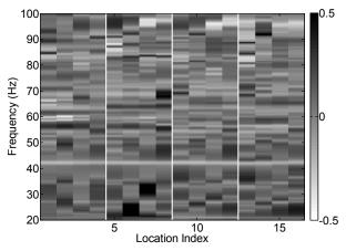
Fig. 3.7 Simulated error agreement as a function of frequency and location index (see Fig. 3.5), as a result of a single corner subwoofer configuration
