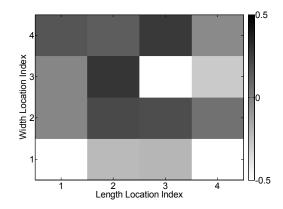
Fig. 3.12 Measured mean error agreement as a function of location index (see Fig. 3.5) where point (1, 3) is closest to zero (perfect error agreement), as a result of a single corner subwoofer configuration
