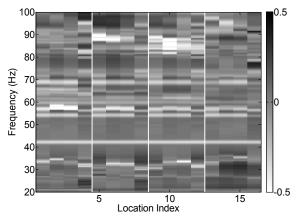
Fig. 3.10 Simulated error agreement as a function of frequency and location index (see Fig. 3.5), as a result of a two-subwoofer sidewall midpoint configuration
