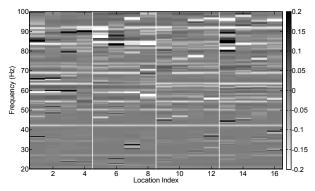
Fig. 3.18 Change in phase error due to simple average equalization (negative = improved response)
