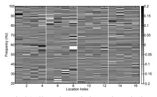
Fig. 3.17 Change in magnitude error due to simple average equalization (negative = improved response)
