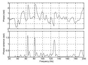
Fig. 3.4 Comparison of the ideal phase response (top) and its phase variance (bottom) for a 10-cycle tone burst
