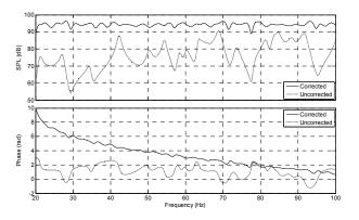
Fig. 3.15 Comparison of corrected and uncorrected magnitude (top) and phase (bottom) responses due to a single-point inverse-filter equalization procedure
