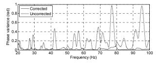
Fig. 3.16 Comparison of corrected and uncorrected PV due to a single-point inverse-filter equalization procedure
