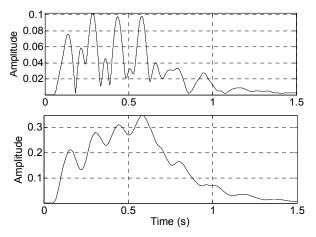
Fig. 3.9 69 Hz tone burst amplitude envelopes (10 cycles, 4 repetitions) at location index (1, 4) (top) and (3, 3) (bottom) relating to the data in Figs. 3.7 & 3.8
