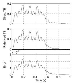
Fig. 3.1 80 Hz tone burst measurements (amplitude envelopes) for (top) direct measurement, (middle) impulse response-derived tone burst where (bottom) is the error between the top two data sets
