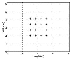
Fig. 3.5 Measurement point configuration in the University of Essex Audio Research Laboratory
