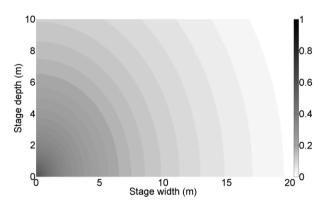
Fig 4.1 Received signal strength (RSS) map for a single antenna at (0.0 m, 0.0 m, 2.0 m) and a calibration location (0.5 m, 0.5 m, 1.6 m)
