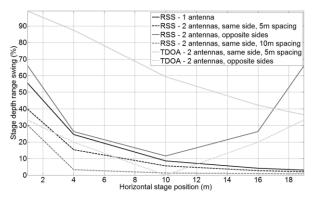
Fig 4.8 calculated range percentages for various horizontal locations using various system configurations (anechoic environment)
