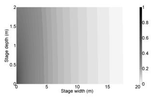
Fig 4.2 Received signal strength (RSS) map for an antenna (0.0 m, 0.0 m, 2.0 m) and calibration location (0.5 m, 0.5 m, 1.6 m), over the first 2 m of stage depth
