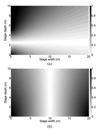
Fig. 4.7 TDOA map for two antennas at (0.0 m, 0.0 m, 2.0 m) and: (a) (0.0, 5.0, 2.0) or (b) (20.0, 0.0, 2.0)
