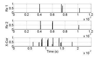
Fig 4.6 Example of cross-correlation based on received signals at two antennas located at (0.0 m, 0.0 m, 2.0 m) and (0.0 m, 5.0 m, 2.0 m) and a transmitter located at (12.0 m, 1.4 m, 1.6 m) with three reflections corrupting the received signals
