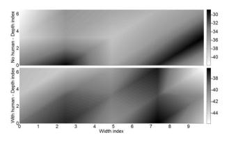
Fig 4.9 Received signal strength (RSS) measurements for two antennas at (0.7 m, 0.0 m, 2.0 m) and (9.1 m, 0.0 m, 2.0 m) with no human interference (top) and with human interference (bottom)
