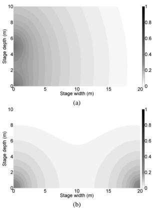
Fig. 4.3 Received signal strength (RSS) map for two antennas at (0.0 m, 0.0 m, 2.0 m) and: (a) (0.0, 5.0, 2.0) or (b) (20.0, 0.0, 2.0), with calibration locations (0.0 m, 2.5 m, 1.6 m) and (10.0 m, 0.0 m, 1.6 m), respectively
