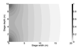
Fig. 4.4 Received signal strength (RSS) map for two antennas at (0.0 m, 0.0 m, 2.0 m) and (0.0, 10.0, 2.0), with calibration location (0.5 m, 0.5 m, 1.6 m)
