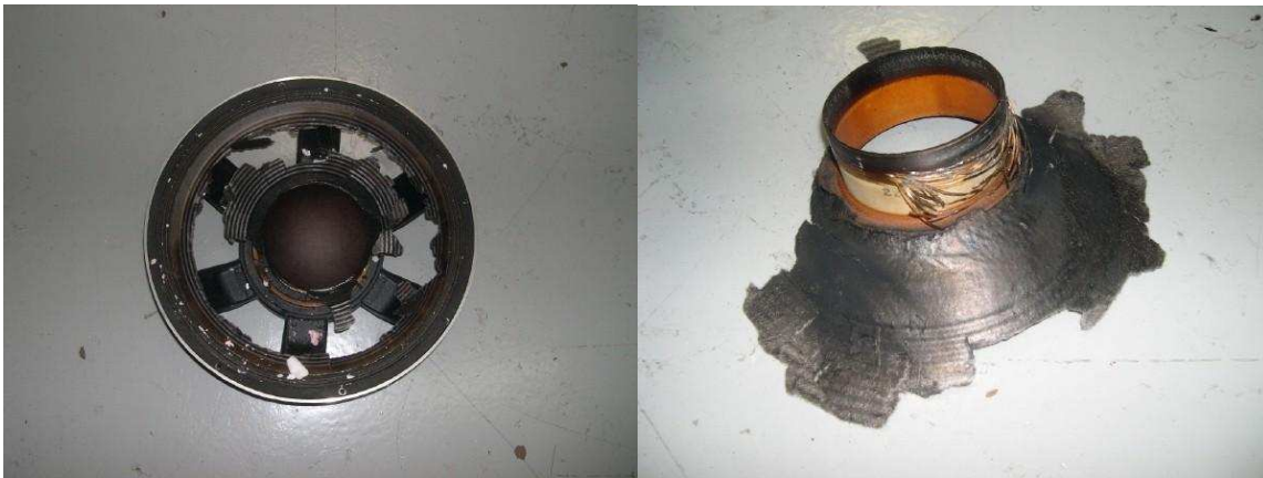
Images 4.1 & 4.2: Driver after voice coil temperature induced combustion
