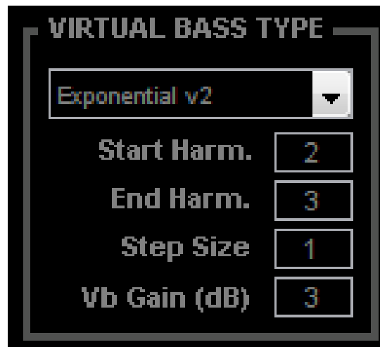
Figure 4 Layout of the VIRTUAL BASS TYPE section
